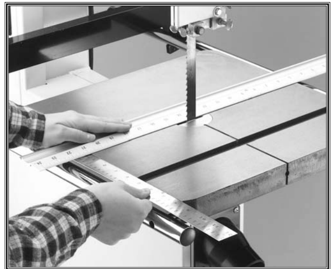
Figure 45. Squaring miter slot to blade.
